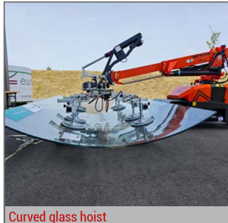
Curved glass hoist
