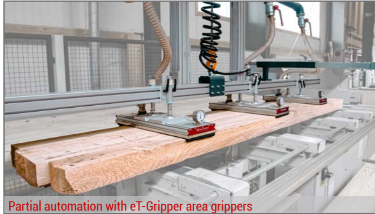
eT-Gripper area gripper in a fully automated system
