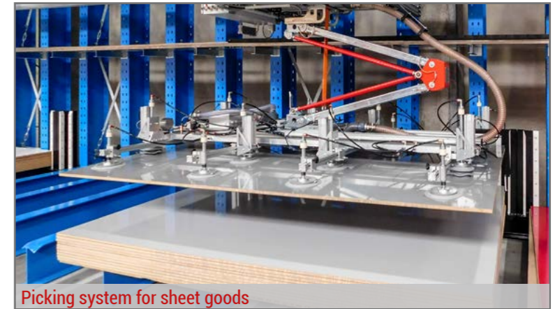
With surface grippers, even heavily structured wood, including sawdust, is no problem
