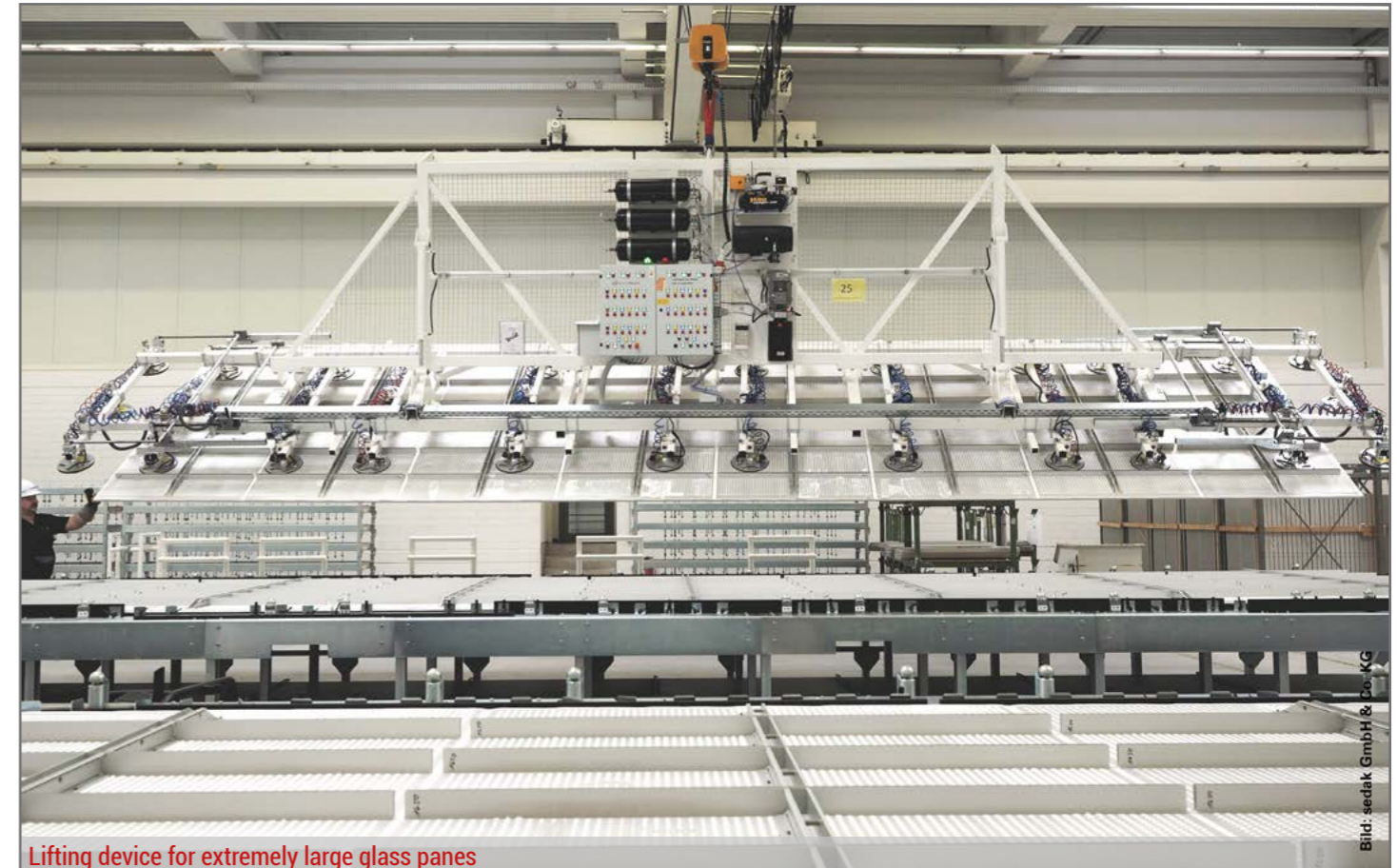
Lifting device for extremely large glass panes
