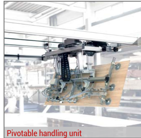
eT-Gripper area gripper in a fully automated system
