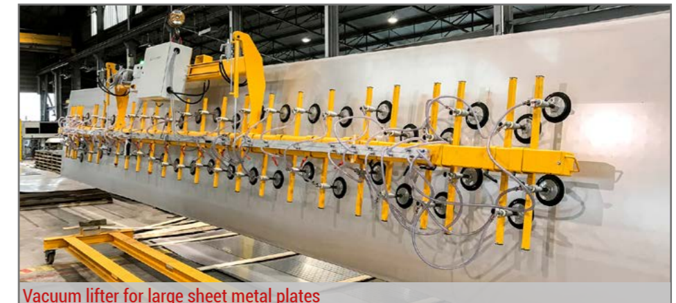
Vacuum lifter for large sheet metal plates
