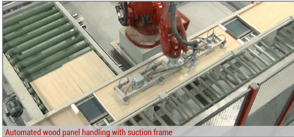
Partial automation with eT-Gripper area grippers
